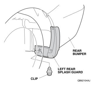
9. Repeat steps 5 through 8 to install the right rear splash guard on the right side of the vehicle.
